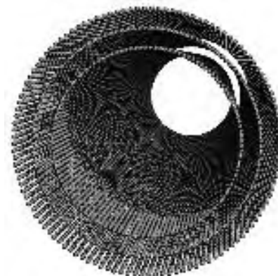
Figure 3.1b Schematic of a multi-walled carbon nanotube (MWNT)
